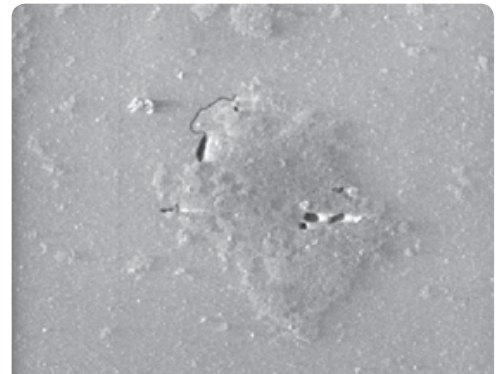
Surface alteration after ageing test of a not controlled thermal forming process
